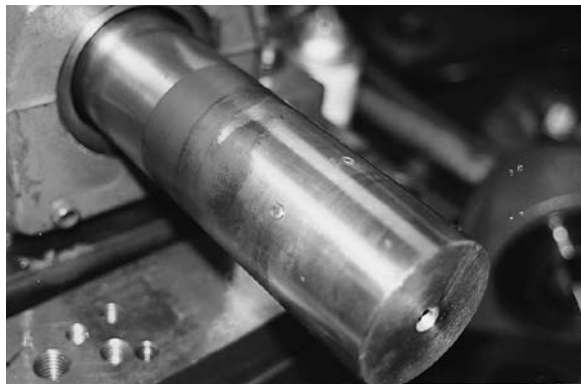
Typical fretting corrosion and shaft damage with eccentric collar bearing. Bearing quite often is "frozen" to shaft
