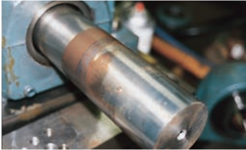
Setscrew Bearing after 500 hours
