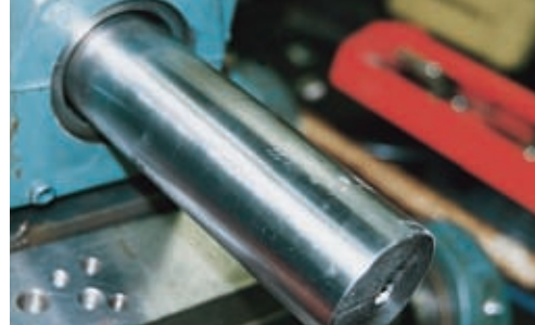
IMPERIAL bearing after 2500 hours
